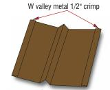
Figure 13d: **Roof Valley Flashing Detail**
