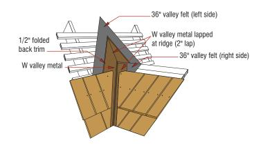
Figure 13b: Typical Saddle Flashing Detail
