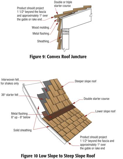
**Transition Detail - Certi-label<sup>®</sup> shakes** (Certigrade<sup>®</sup> shingle application is similar but without felt interlay)
