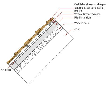
Figure 18: Specialty Roof Deck-Vented Roof
