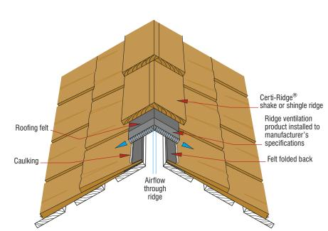
**Figure 16: Ridge Ventilation Detail**
