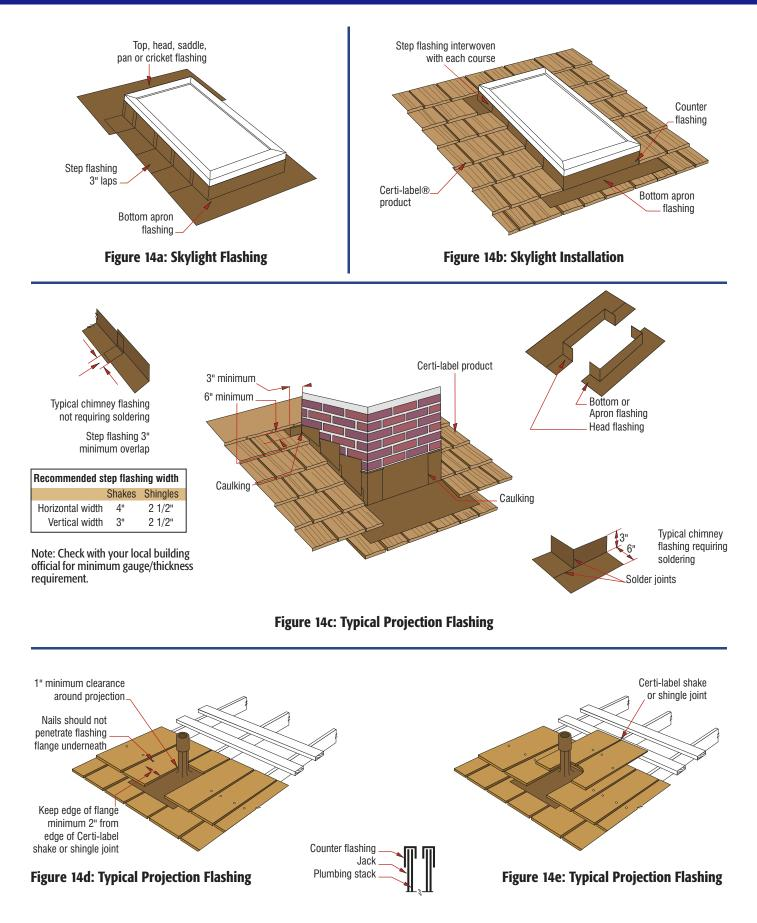
Figures 14a-14e: Flashing Details for Typical Roof Projections
