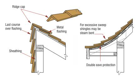
Figure 11: Apex Roof Juncture
