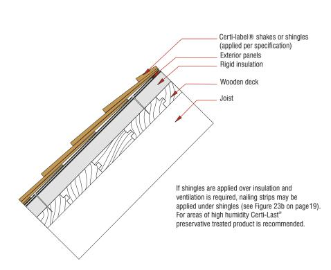
Figure 19: Specialty Roof Deck-Panels Over Insulation
