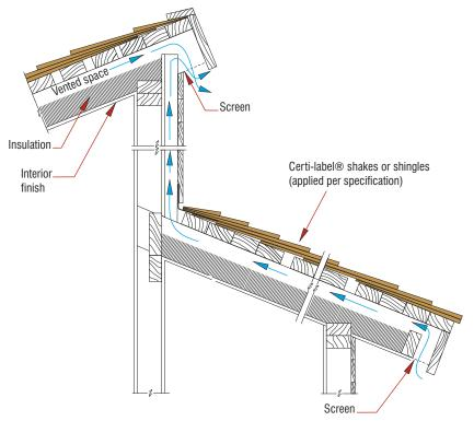
**Figure 22: Half Monitor Roof**
